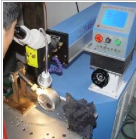
激光焊接设备，将表壳及接头焊在一起。 Laser welding equipment, to weld connection and case together;
